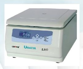
Easy to use, many kinds of rotors. Fast Acceleration /Deceleration function. 9 Acceleration (ACC) and 10 Deceleration (DEC) profiles. Microprocessor control, LCD display, DC brushless motor. It can store 25 different programs in memory. Electronic door interlock and stainless steel chamber. Special button for short centrifugation. The parameters can be changed freely during the run. The protection function of imbalance.e.
